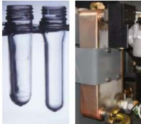
Left: Preforms made from pressed plastic powder.
